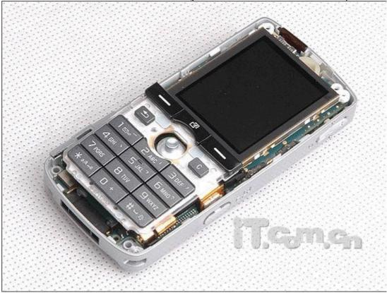
Next, to remove the keypad plate and black plastic backing, gently lift it up like you're opening the lid to a chest. You'll see the PCB connector clearly now, so using a small flat screwdriver, unplug it and lift the assembly free.
