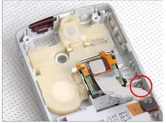
Now on with the camera - you must remove the little sticky camera switch (circled) and the sticky flash LED piece (arrowed) from the chassis. Just gently peel them off. Don't get your fingers all over the sticky sections as you'll need them to remain sticky to go back on again!
