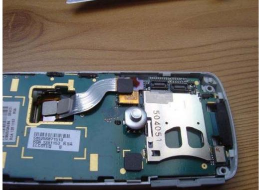
Before we do this, unplug the camera from the PCB and feed this connector through the hole in the PCB (pictured far left of this image), as you lift it free.
