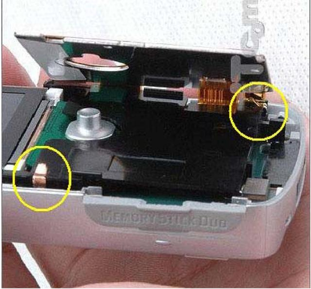
This is the assembly removed. You can clearly see a) one of the brass-like clips, b) the PCB connector and c) the camera button. There is NO need to separate the keypad plate from the backing plate as in this image. This is just for illustration purposes only.
