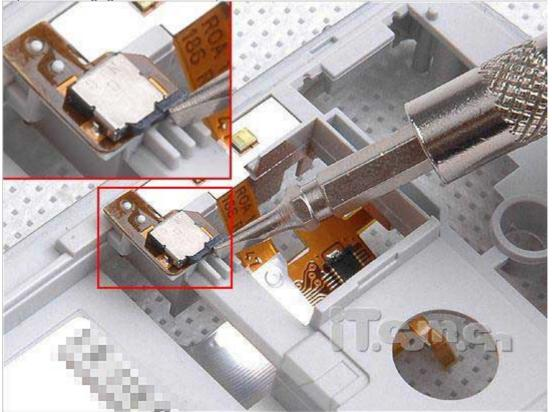
This is an image of the speaker assembly. It is gently prised and peeled out of the chassis as it has a sticky section around the speaker itself, holding the assembly in place.
