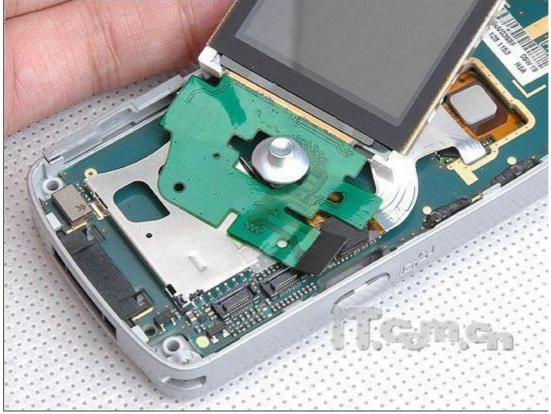
To remove the PCB itself, use a small flat screwdriver and gently work your way around the chassis and prise the PCB free. Now, working from the top of your phone, lift it and pull it out from the base connector.
