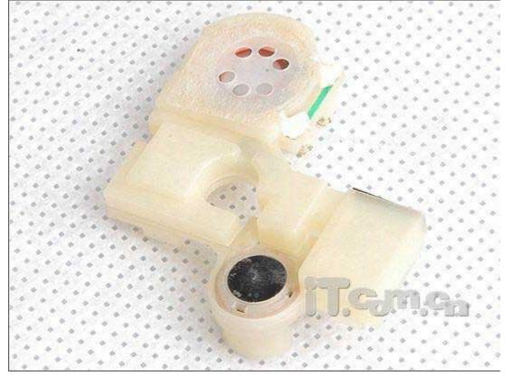
The antenna assembly proved a bit of a bugger to get out. What I found easiest was, from the other side to that shown in the image, I used a flat blade screwdriver and gently eased the 2 clips (which form part of the white plastic) out, to release the assembly from the chassis.
