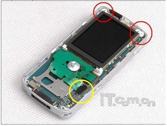
Then, easing it over the joystick, lift the screen free.
