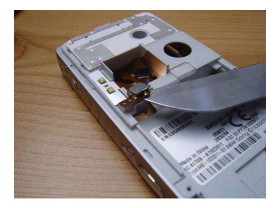
WARNING: Be extremely careful of this switch as it's the 'trigger' for your camera! Don't force it in any direction. (When putting on the phone back cover on later, I opened the lens cover first so as to not interfere with the switch on re-assembly. Close the lens cover once all the clips have engaged in the cover).
